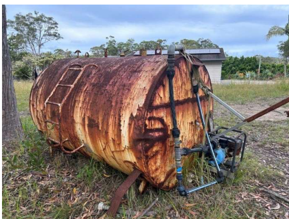
An old liquid storage tank present in the south-west corner of the site. It is unknown what liquids were stored in the tank. No evidence of hydrocarbon storage was observed at the time of the field investigations.
